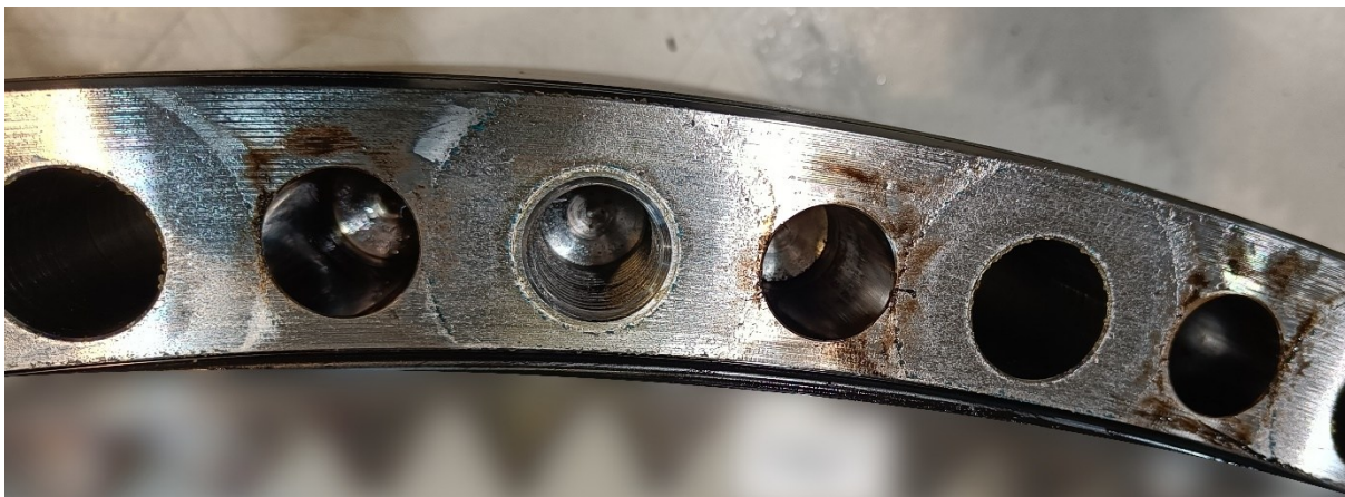
Figure 7: Condition of flange connection after second test, with friction improvements.
