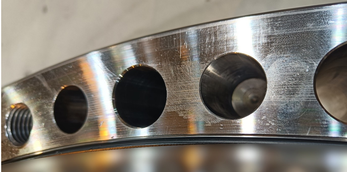
Figure 6: Condition of flange connection after first test.
